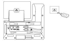
Note: The USB port can also be used to connect other USB devices, such as EXP50, USB headset and so on.
